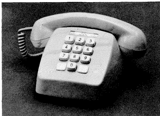
Figure 9—Push-button subscriber station.
