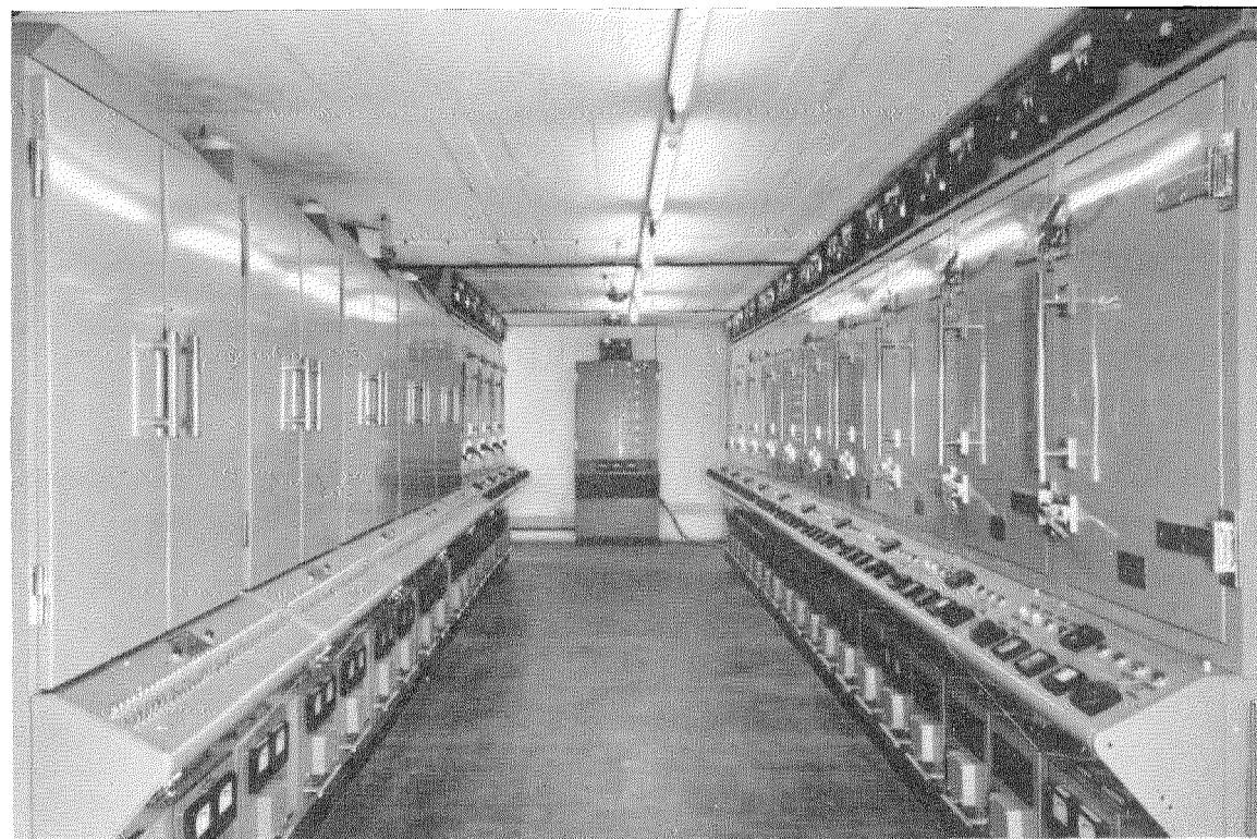
Figure 4—Equipment for reliability and life tests of capacitors, transistors, and diodes.
