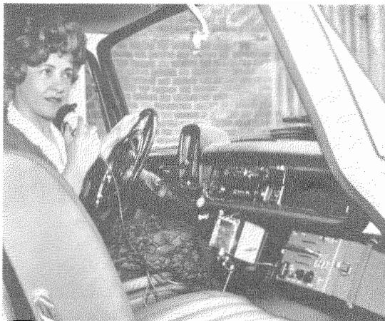
Figure 15—Mobile radiotelephone installation in a Paris taxicab.
